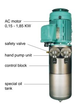
on the command. The motor driven pump starts delivering hydraulic fluid through the special control block and pressurizes the cylinder from the left or the right hand side.
