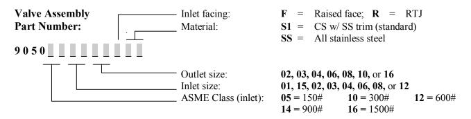
Standard assembly includes **regulator**, **pressure gage**, and **block valve** for dome gas supply from customer-furnished gas source. Specific components and supply configuration to be selected for each application; contact factory for details.
